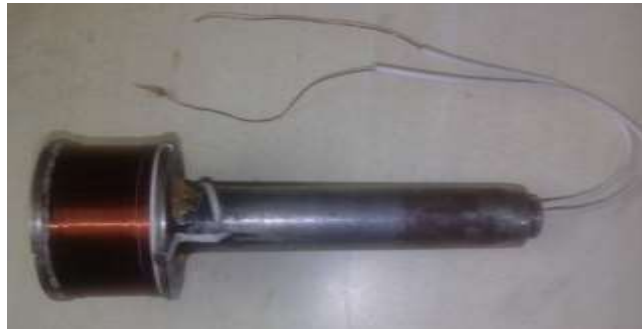
Fig. 6 Magnetic circuit of MR damper
