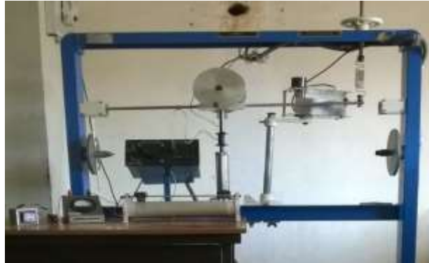
Fig.8 Experimental setup for MR damper testing
