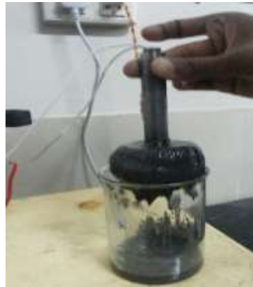
Fig.4 Actual schematic of MR fluid after applying magnetic field
